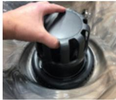
Pull Up to Remove Floater Assembly
