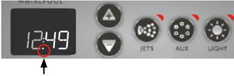
Enter the program menu by holding down the **PROGRAM/LIGHT\*** button for 5 seconds. The display will show the current clock setting with the hour flashing. Your system is set on 12-hour time.
