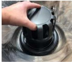
Pull Up to Remove Floater Assembly
