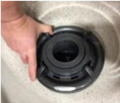
Twist Lock Ring Counter-clockwise to Remove Floater
