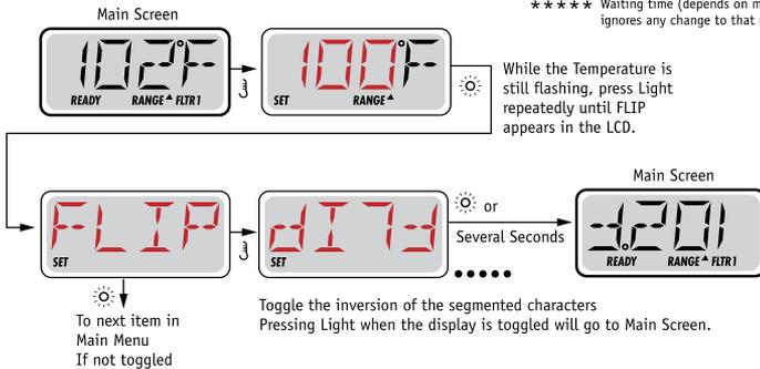
**NOTE:** Some panels may have a dedicated **FLIP** button, which allows the user to flip the display with a single button-press.
