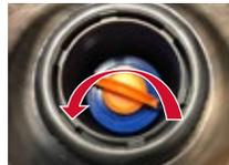
*Turn Filters Counter-clockwise to Remove*
