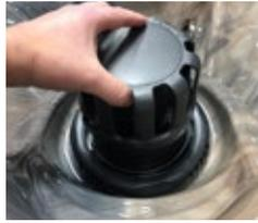
Pull Up to Remove Floater Assembly
