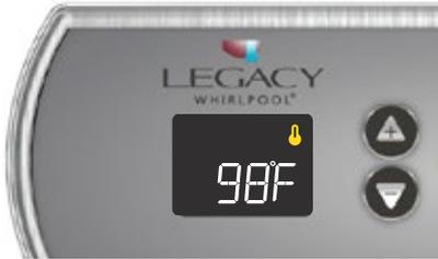
The temperature shown on screen is the current water temperature. Use the **UP** and **DOWN** arrow buttons to set the desired temperature. The temperature setting will be displayed for a few seconds before confirming your new selection.
