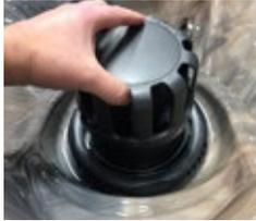
*Pull Up to Remove Floater Assembly*
