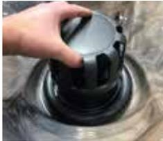
*Pull Up to Remove Floater Assembly*
