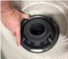
*Twist Lock Ring Counter-clockwise to Remove Floater*
