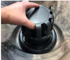
*Pull Up to Remove Floater Assembly*
