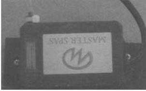
**6. OZONATOR.** Your optional ozonator will operate in conjunction with your filtration system. It will deactivate when any other control function is manually activated and will reactivate after one hour of inactivity.
