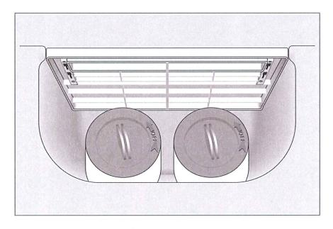
To service and clean your filter elements, turn counter-clockwise 6-8 revolutions. To reinstall, turn clockwise 6-8 revolutions. For more complete instruction, see "*To Clean Your Filter Elements*," p. 19.
